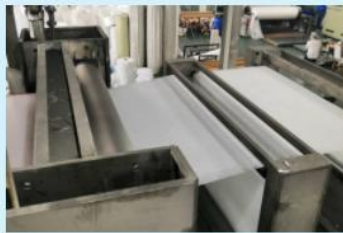
4. The stretched superfine fiber is transferred to the web former. Forming the embryonic form of non woven pp meltblown fabric
