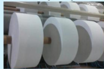
6. Cut off the edges on both sides, eventually become a non woven coiled material
