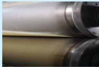
5. The non woven fiber web transferred to calender by net screen and will be pressed by calendar, rolling up the completed meltblown fabric rolls
