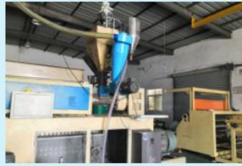
2. Polypropylene is conveyed to the inside of the machine body and melt
